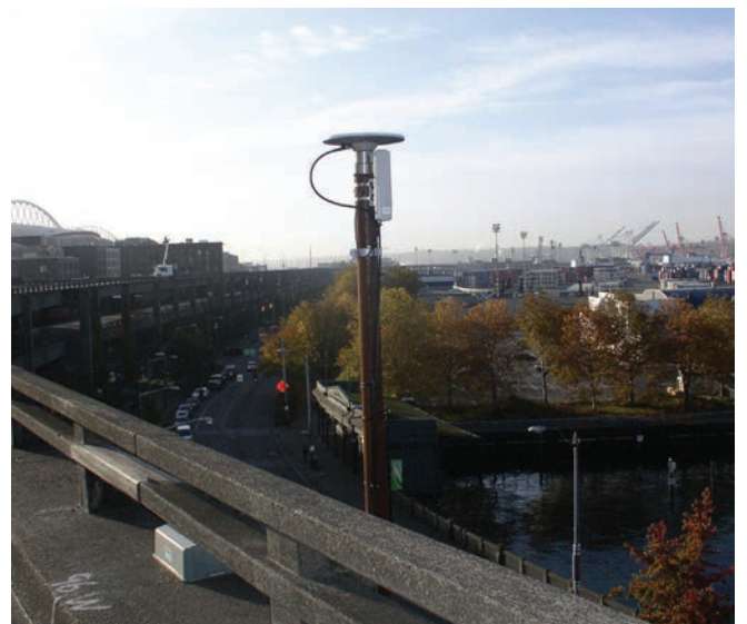
A monitoring device installed on the viaduct. Removing cars will make it easier for crews to monitor and respond to any movement they might detect.
